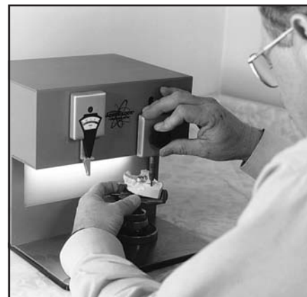
Fig #4: The Retentoscope accurately measures the depth of the abutment's undercut.
