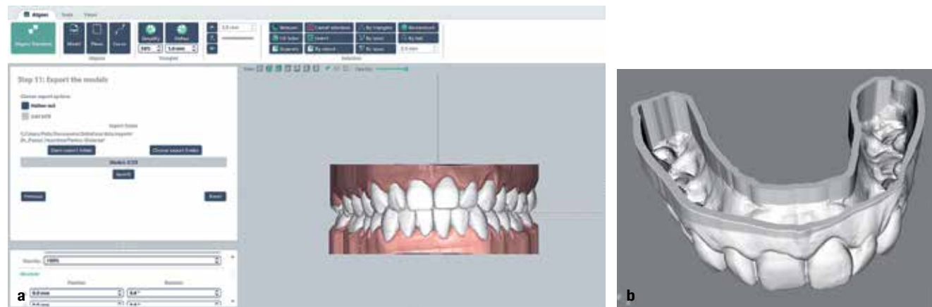
Fig 10-22 (a) Exporting the models to fabricate a hollow dental model. (b) Hollow dental model.
