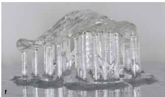
Fig 6-33 (cont) (d and e) Virtual placement of the OrthoEasy Pal microimplants with the help of a blade placed on a low-speed hand-piece. (f) The surgical splint printed on the 3D printer's platform. (g) The surgical splint after alcohol rinsing and UV curing.
