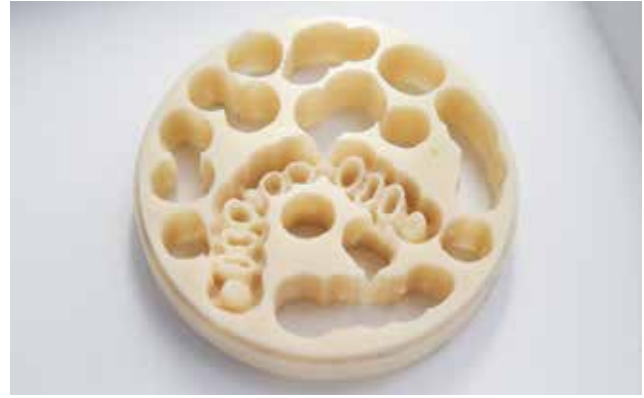
Fig 5-14 The dimension of the milling disk is not suitable for creating most orthodontic appliances.
