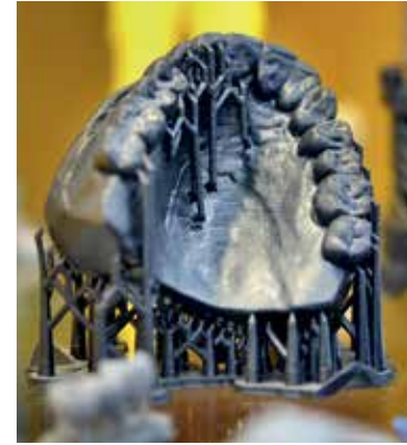
Fig 4-4 3D-printed object showing printing supports in place.
