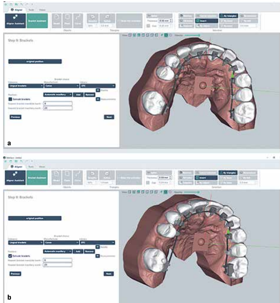
Fig 8-26 Lingual orthodontic treatment using the customized bases option. (a) Automatic positioning of the brackets. (b) Extrusion of the bracket bases.
