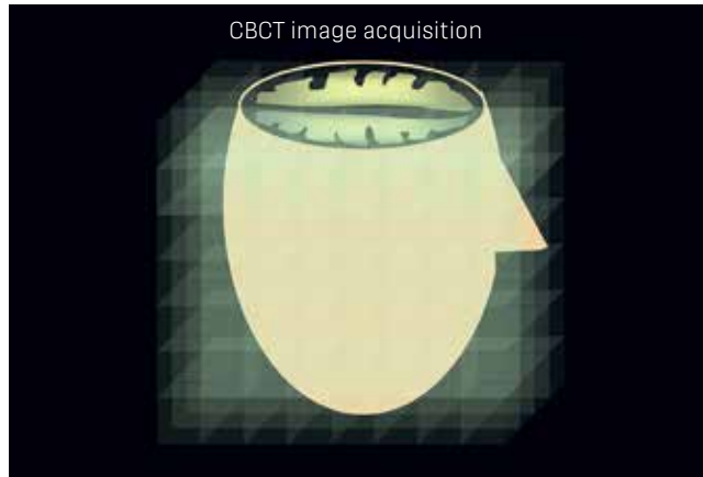
Fig 2-3 The moment a region of interest is determined, this area is “split” in numerous small fictional cubes from which the detector of the scanner will collect attenuation data; these cubes, known as voxels , are of a known spatial location and are assigned a shade of gray after the data are processed. This composite of voxels forms the 3D volume.
