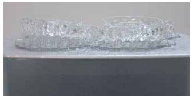
Fig 11-15 The indirect transfer trays printed on the 3D printer platform.
