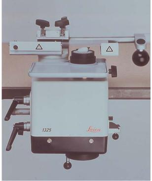
Figure 1.8 Leica 1325 freezing microtome
