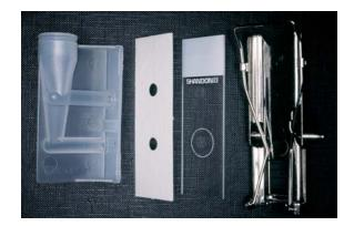
Figure 9.12 Cytocentrifuge chamber components. Suction chamber, filter card, glass slide and spring clip prior to assembly
