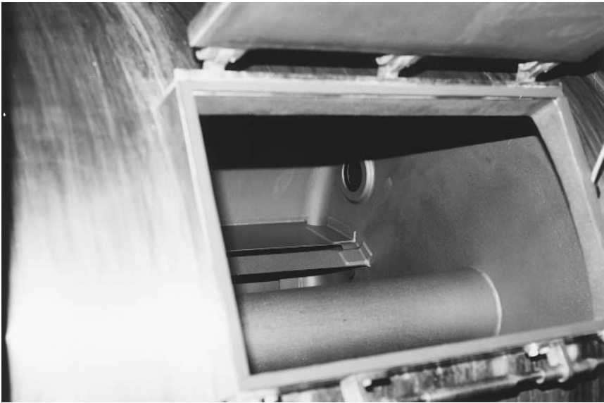
Figure 11 Interior view of a batch churn showing vanes on outer edge, inspection window, and center tube which can have chilled water circulated through it to control product temperature. Butter is removed by one of two ways: (a) manually with metal scoops or (b) by dumping the butter into a boat (hopper) positioned beneath the churn. The boat is then wheeled to the packaging area.
